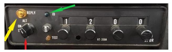
Once the Avionics Master is turned on the transponder should power up as we generally leave the power/selector switch(RED arrow) in the ALT(altitude encoding) position.
